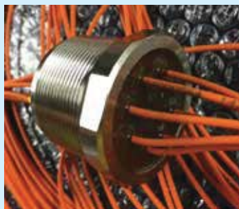
Even test connectors must be potted to protect them from pressure differential and water ingress.
