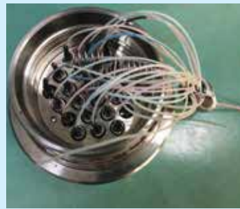
There's no room in the connector back shell for slack. No mistakes allowed!
