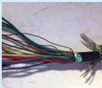
Here's a close up of steel-wrapped fiber cable used in offshore technology.
